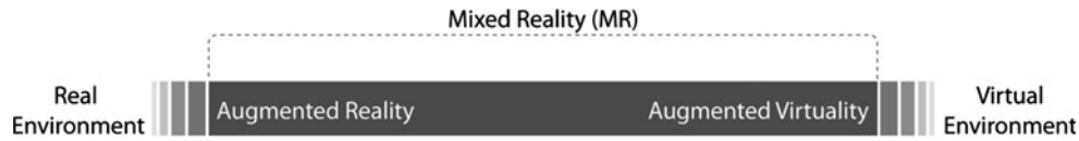
Fig. 1 Virtuality continuum defining the possibilities of the mixture of real-world and virtual-world objects (modified from Milgram and Kishino's 1994 study)
